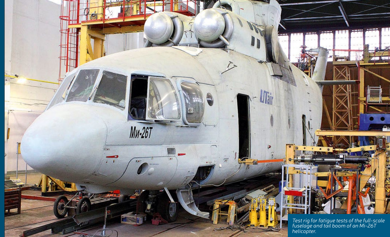
Arrangement of the test rigs for an Mi-26, Mi-38 and Ka-62 in the AVIATEST Research and Testing Centre.
