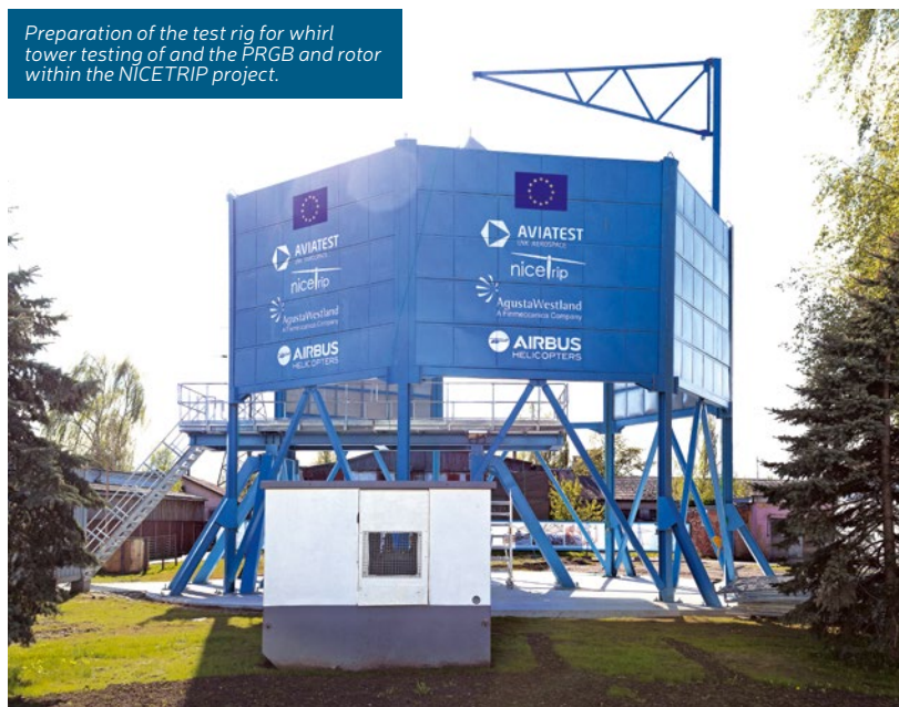
Test rig for testing gears and transmissions of the helicopter.
